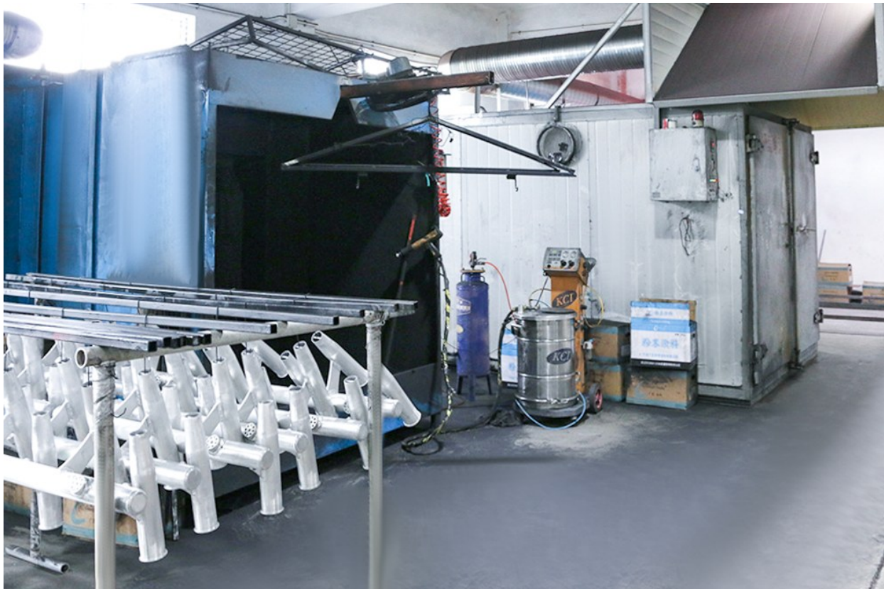
nbfeiyu powder coating workshop for finished metal parts.
