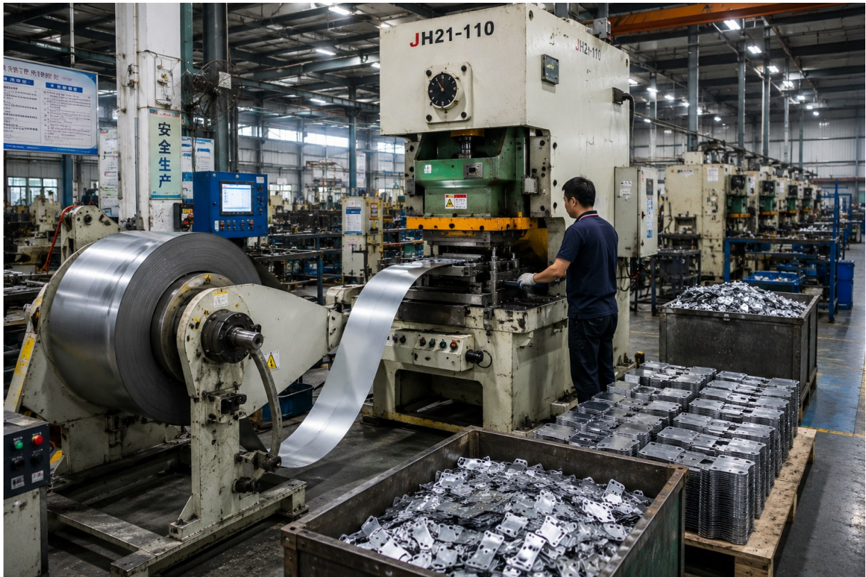
Coil-fed stamping press producing sheet metal parts in the nbfeiyu factory workshop.
