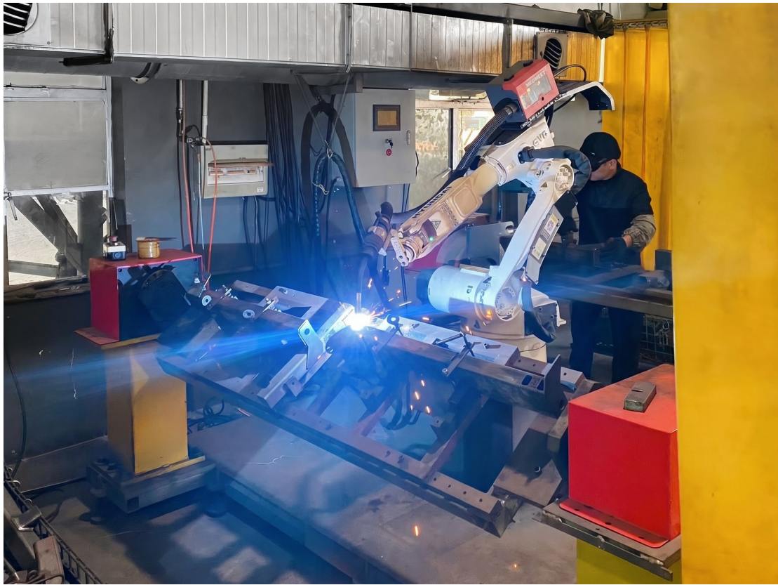
nbfeiyu robotic welding cell for metal frame production.
