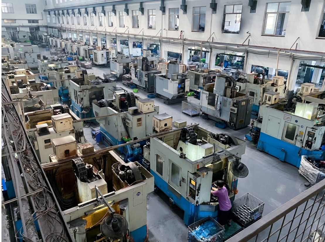
nbfeiyu CNC machining workshop with multiple machining centers.
